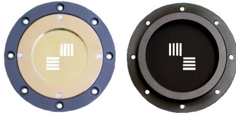
Fig. 4.19. Photo of a multiply 4-bar target used for MRTD measurement from two sides.
