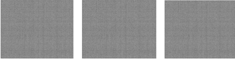
Fig. 3.24. Three neighbor images of uniform target generated by a thermal camera of dominant high frequency spatial noise.
