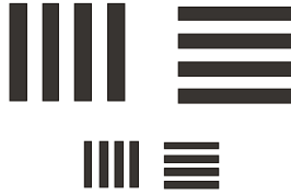
Fig. 5.8. Exemplary multi pattern target (black color-holes, white color – metal plate).
