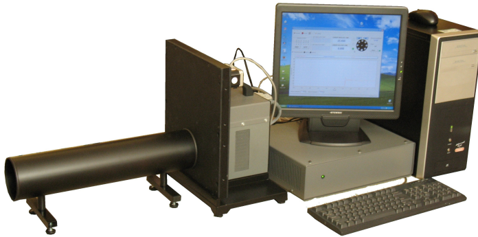
Fig. 4.7. Photo of the SAFT variable target/distance measuring system.
