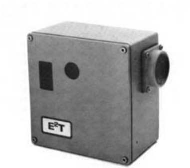
Fig. 19. Dualband narrow-band pyrometer: DICHROMA manufactured by E 2 T ®
