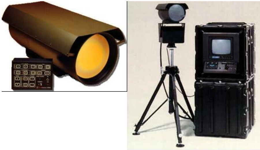
Figure 1. Exemplary Gen 1 thermal camera: LORIS (courtesy of FLIR Inc)
