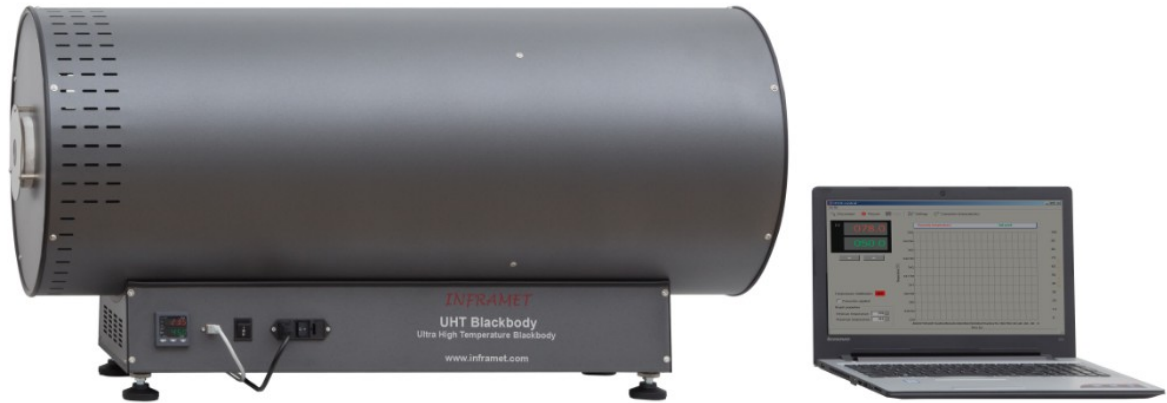
Fig. 1. Photo of the UHT-38D-1500 blackbody
