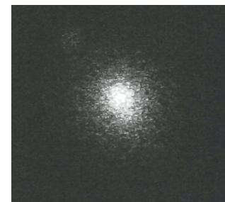
Fig.4. Image of illuminated field by laser illuminator of poor illumination uniformity
