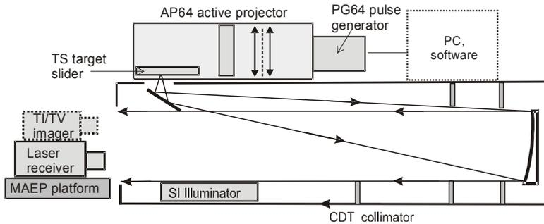
Fig. 2.. Block diagram of L64 test system
