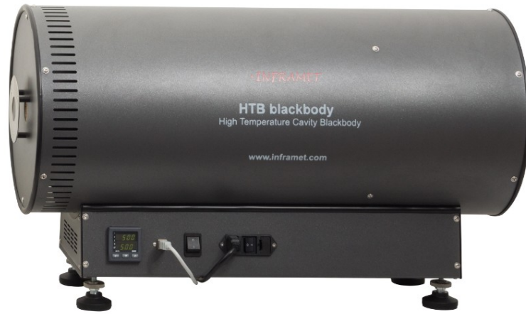
Fig. 1. Photo of the HTB-35D-1200 blackbody
