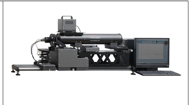
Fig. 2. FT-I configuration of FT test system (measurement of image quality parameters)
