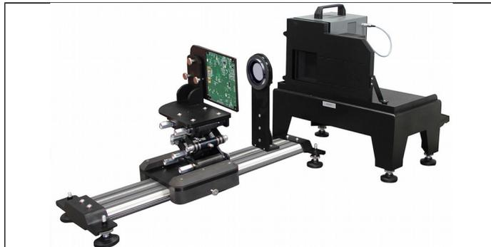
Fig. 1. FT-N configuration of FT test system (measurement of noise/responsivity parameters in static flood mode)
