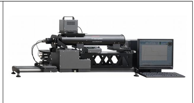
Fig. 2. FT-I configuration of FT test system (measurement of image quality parameters)
