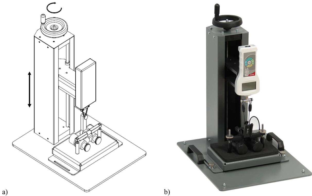
Fig. 1. FORK test station: a)block diagram, b)photo
