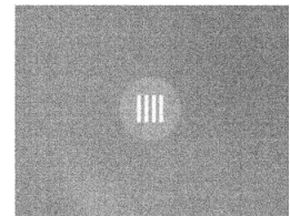
Fig. 3. Image of a 4-bar target (projected by DT 150 system and generated a by thermal imager)
